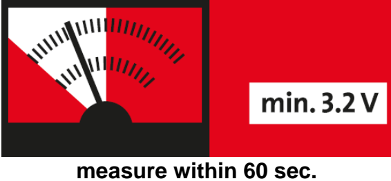
Figure 6: Battery Voltage Measurement
