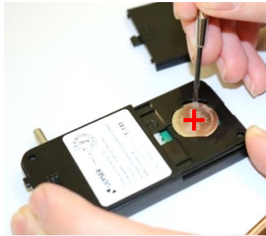
Figure 30: Replace the battery
