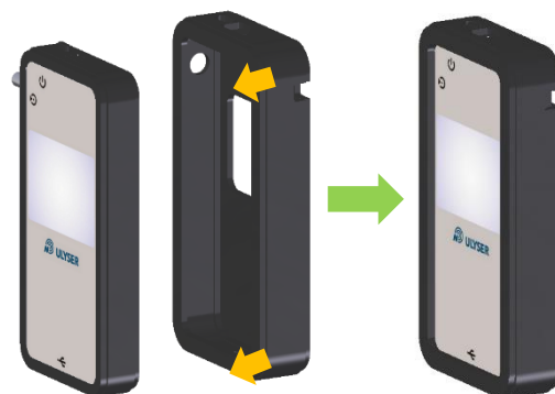
Figure 32: Mount the silicone sleeve
